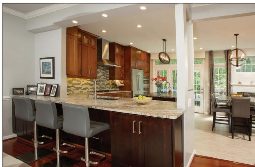
To create an "open" plan in the middle of a three-level townhouse, designers deleted a bearing wall between the kitchen and a formal dining area, insinuating an I-beam supported by concealed vertical shafts to hold up the floors above. The opening made way for a three-seat dining counter that faces in towards the kitchen. The change also allows more natural light from front to back.
